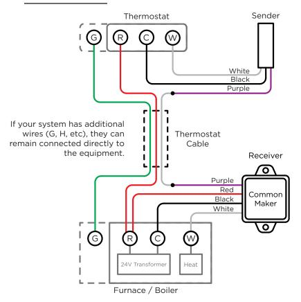
B Dry Contact Switching with Internal Transformer
