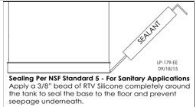
Figure 25 - Sealing the Water Heater for Sanitary Applications
